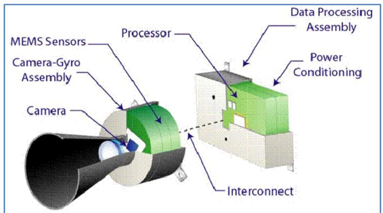
*Compass is built as two separate assemblies, the camera-gyro assembly and the data processor assembly, connected by a wiring harness. The technology uses an active pixel sensor in a wide-field-of-view miniature star camera and micro-electromechanical system (MEMS) gyros. Together, they provide extremely accurate information for navigation and control.*
